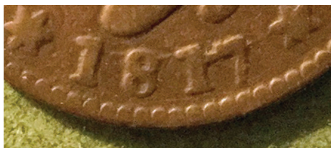
Picture 2-10. Very Early Die State Breaks at the Date (Coin image courtesy Tom Nist)
