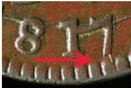
Picture 2-8. Thick 7 / Bottom 7 Breaks – LDS Coin (Coin Image courtesy John Wright)
