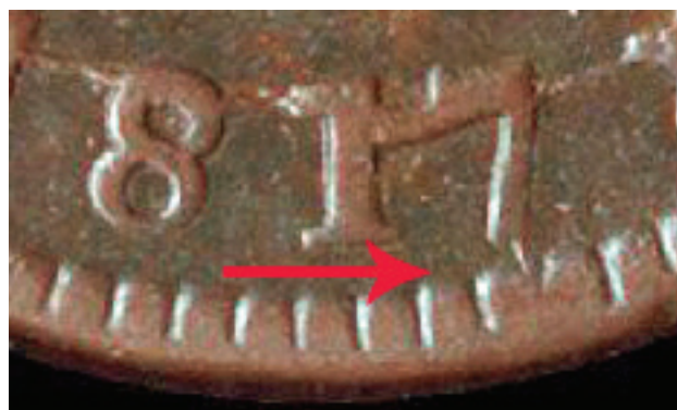
Picture 2-9. Thick 7 / Bottom 7 Breaks – TDS Coin (Coin Image courtesy John Wright)
