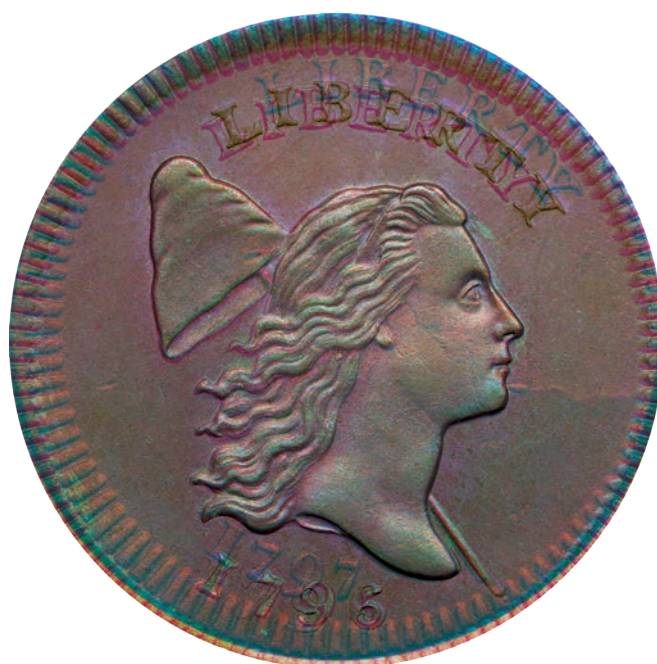
Figure 7. Overlay of obverses from 1795, 1796 and 1797. The entire head and cap match and so were from the same master die. The lettering, date, pole and dentilation were individually engraved in each die.
