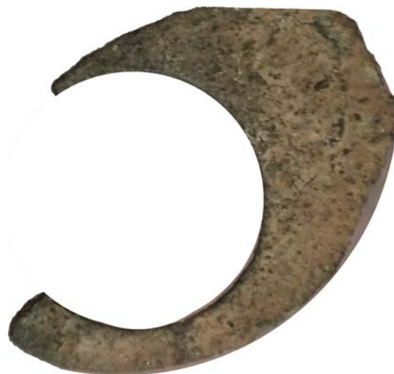
Rolled out cent or token from which a half cent planchet has been cut.
