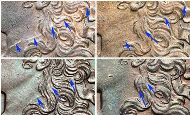
Figure 14. “Hub flaw” and hair engraving of Classic Head half cents. The flaw, actually a flaw in the master die, is indicated by blue arrows in each image. Upper left, 1809 C-4. Upper right, 1809 C-3; much of the flaw has been tooled away. Lower Left, 1826 C-2. Lower right, 1833 C-1; only faint traces of the flaw remain. The hair is strengthened by engraving on the 1826 and 1833 dies.
